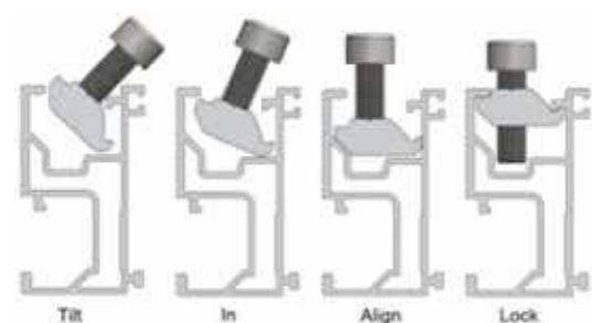
Four Steps to put the tilt-in module into rail easily
