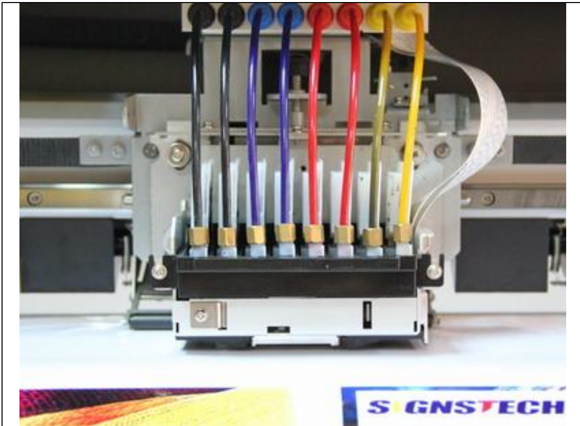
High quality and refined carriage with double sliders on linear rail
