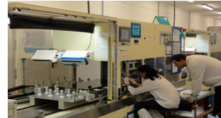
SOF bonding on glass side
