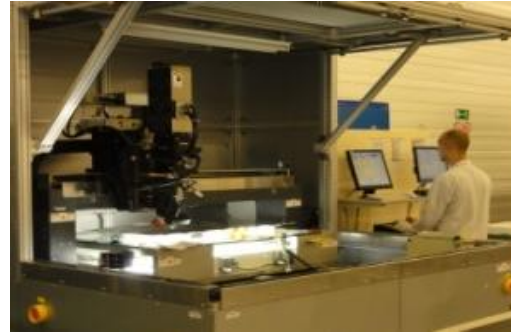
LCD panels repair by using lasers
